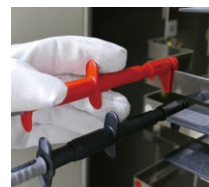
For clamping around the target busbar
